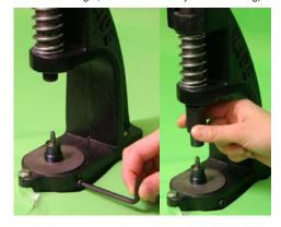
**3. Inserting Grommet Components:** Insert the grommet body into the hole that you pierced into the material previously. Place the grommet washer onto the bottom grommet setting die with embossed side down.
