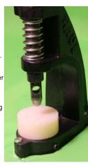
3. Prepare to press Grommets: remove cutter tool & cutting block from the press and put them aside. Insert the bottom die into the base hole and tighten the Allen screw with the included Allen wrench, so that the bottom die will not come out of place. Carefully thread the top grommet die to the press spindle
