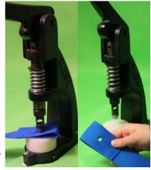
**4. Inserting Grommet Components:** Insert the grommet body into the hole that you cut into the material previously. Place the grommet washer onto the bottom grommet setting die with embossed side down.
