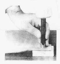
Fold material and mark for location of grommet. Put the cutting block under the mark. Place cutter (a) over mark and strike with mallet to cut hole.
