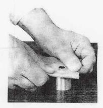
Insert grommet (d) from below, placing it on base (c) so that hole in grommet lines up with hole in base (c). Put washer over the grommet (d) rounded side up.
