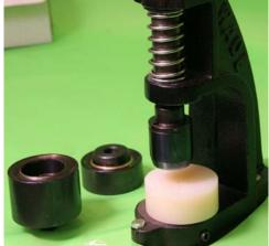
3. Prepare to press Grommets: remove cutter tool & cutting block from the press and put them aside. Insert the bottom die into the base hole and tighten the
